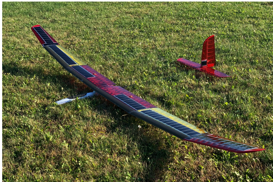
Figure 1: The UIUC-TUM Solar Flyer aircraft shown with solar arrays.
