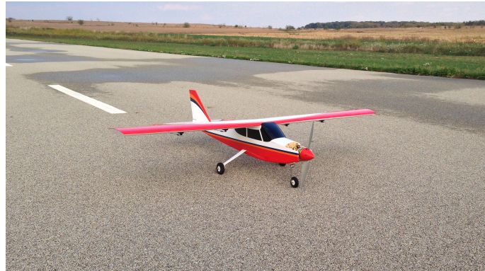
Figure 1. The flight-ready instrumented Great Planes Avistar Elite.
