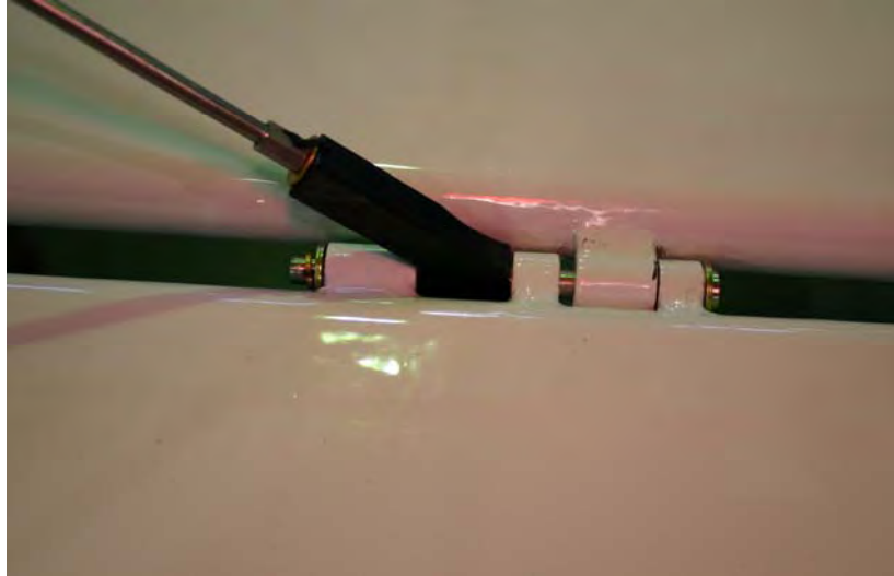
Figure 6.3.5.8 Clevis Pin Installation on Elevator
