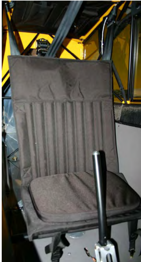
Figure 3 - Rear Sling Seat Installed
