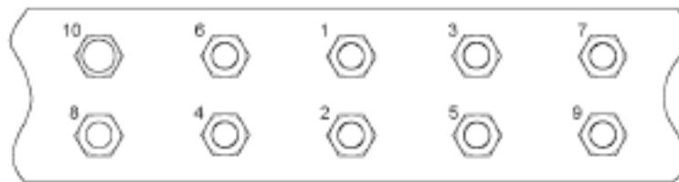
TYPICAL LINEAR PATTERN TORQUING SEQUENCE
