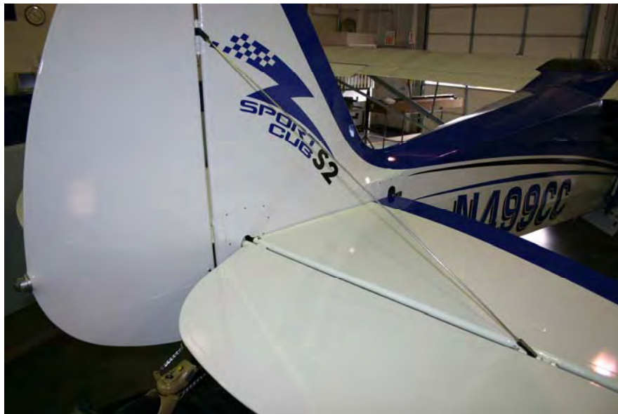
Figure 6.3.5.5 Tail Brace Wires and Elevator Attachment
