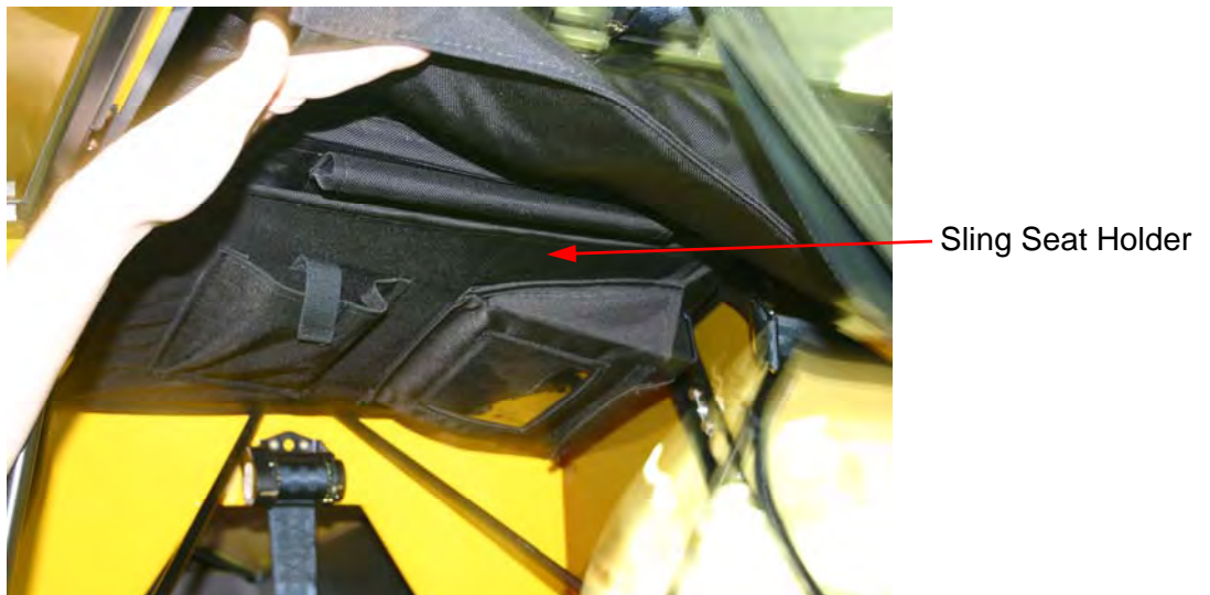
Figure 6 - Rear Seat Stowage in Sling Seat Holder
