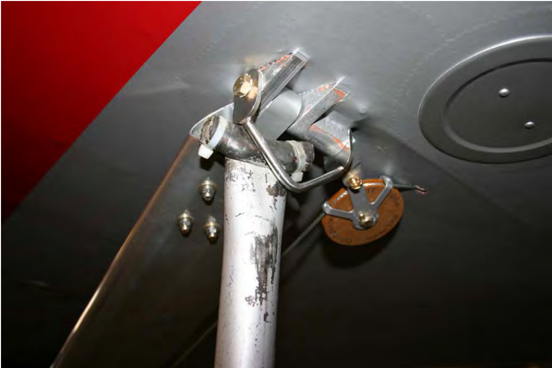
Figure 6.3.2.3: Jacking from the Wing
