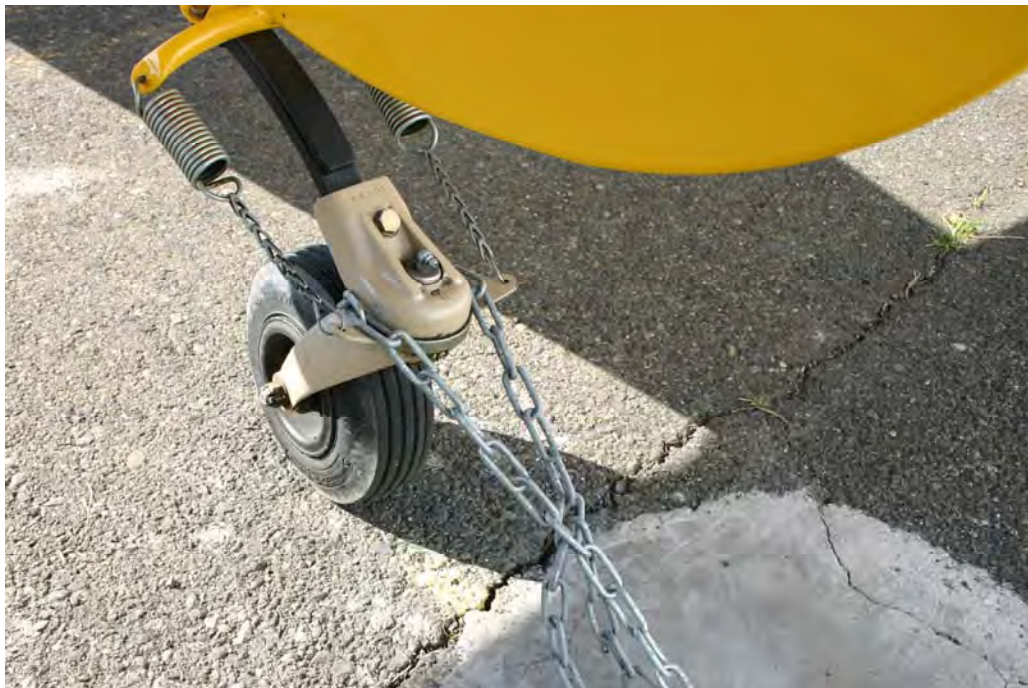
Figure 6.3.24.2: Tailwheel Tie Down
