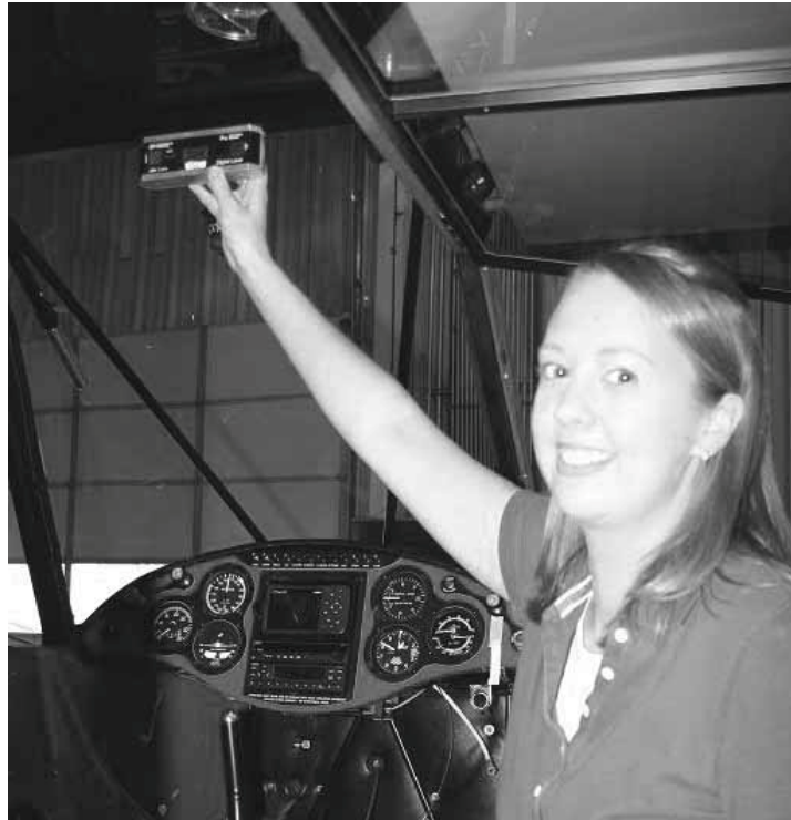
Figure 6.3.22.2: Leveling the Aircraft Laterally
