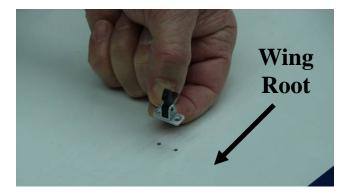
3. Use thick CA on each screw prior to installing to lock screws in place.
