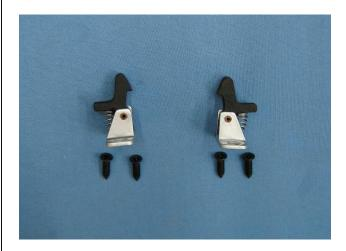
2. Align window latch with predrilled holes in the bottom of each wing. The hook portion of the latch will go towards the wing root.
